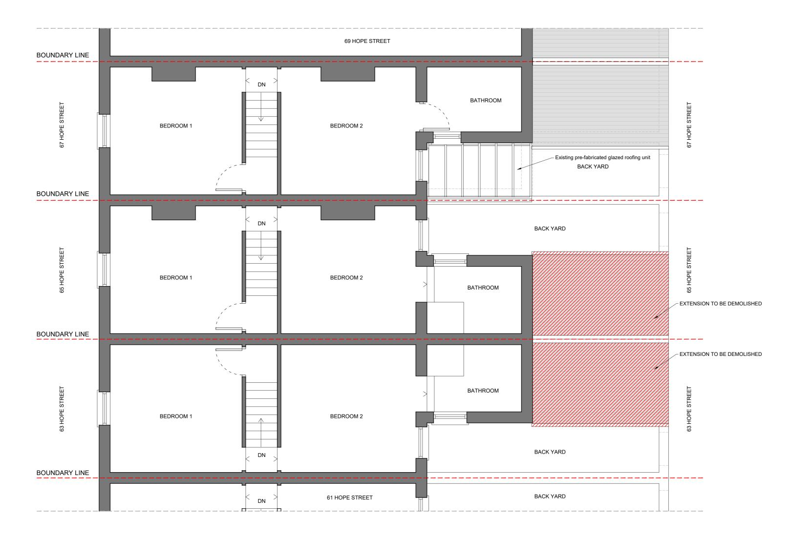
EXISTING FIRST FLOOR PLAN + DEMOLITIONS
