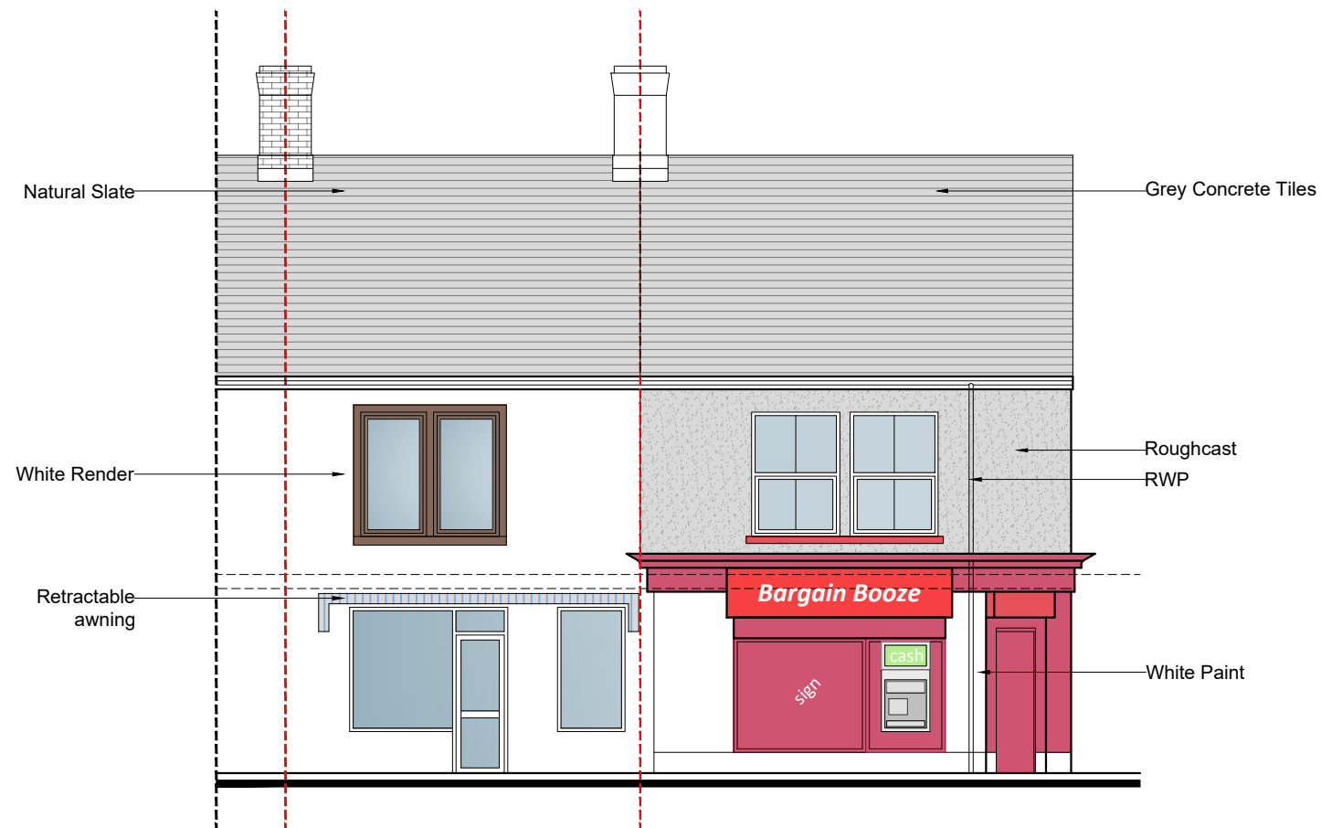
EXISTING SOUTHERN ELEVATION Scale 1:100 @ A3
