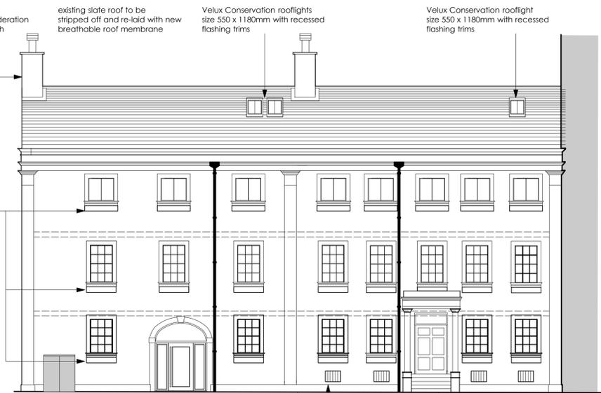
Front Elevation to Harbour new timber double glazed door screen - existing railing to side of ramp removed
