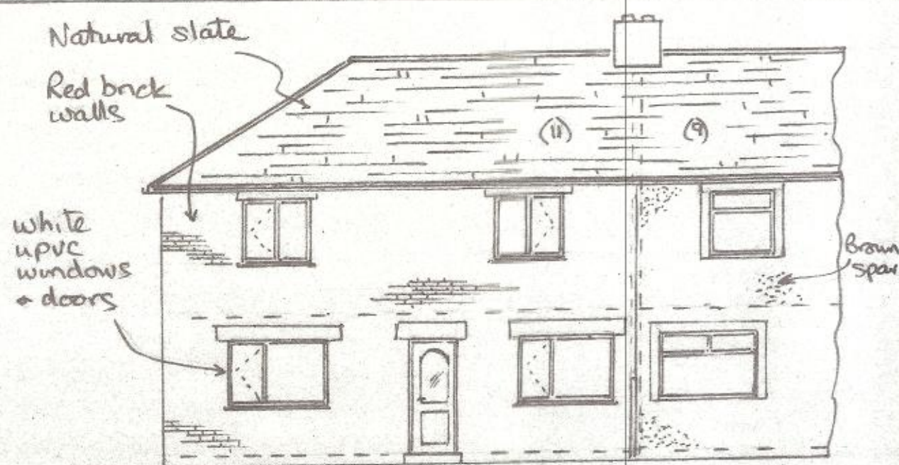
EXISTING NORTH WEST ELEVATION
