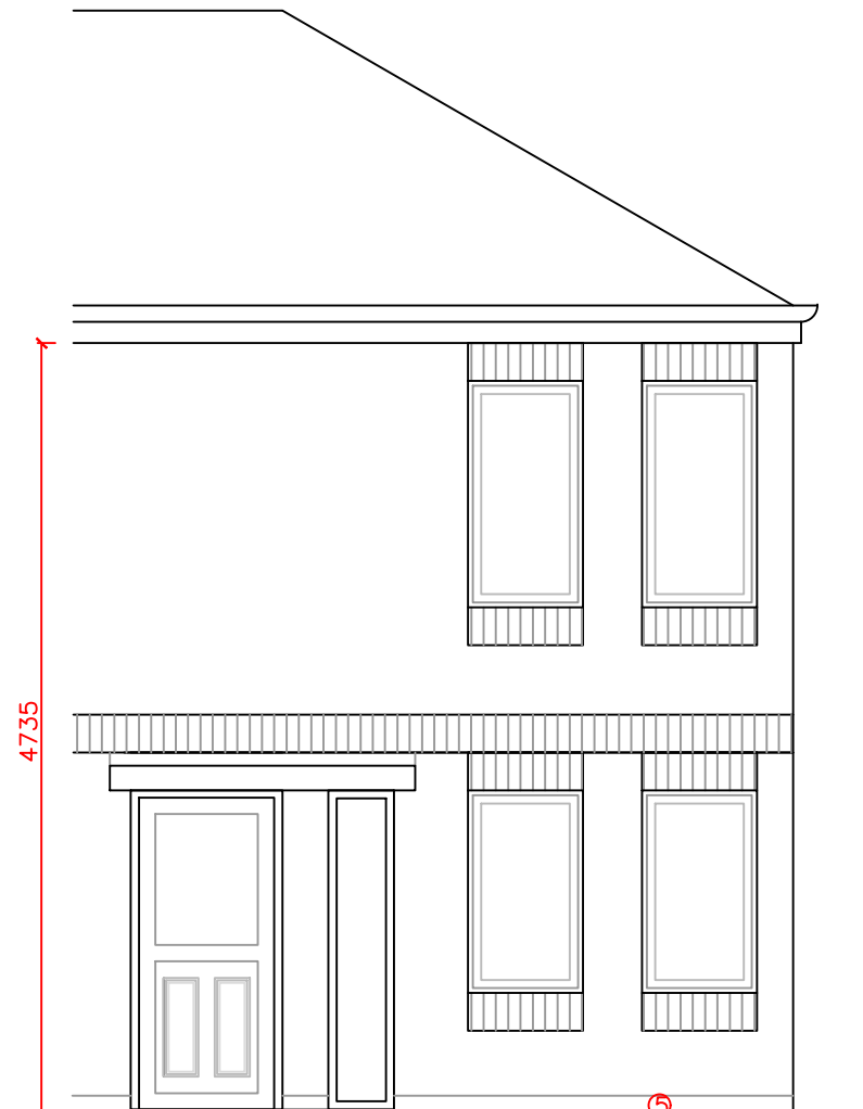
First Floor Rear Elevation (1:50 @ A3)
