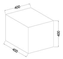
Fill hole with water and allow to drain away naturally. Repeat this process 3 times. If the water does not drain away at all then the sub-grade soil does not have adequate permeability properties
