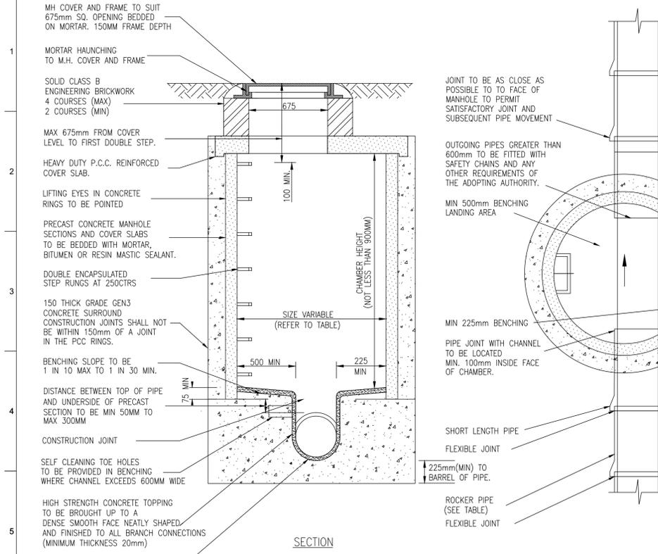
TYPICAL MANHOLE DETAIL - TYPE B
