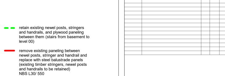
new steel balustrades and handrails to both sides of new steel stair, 900mm
