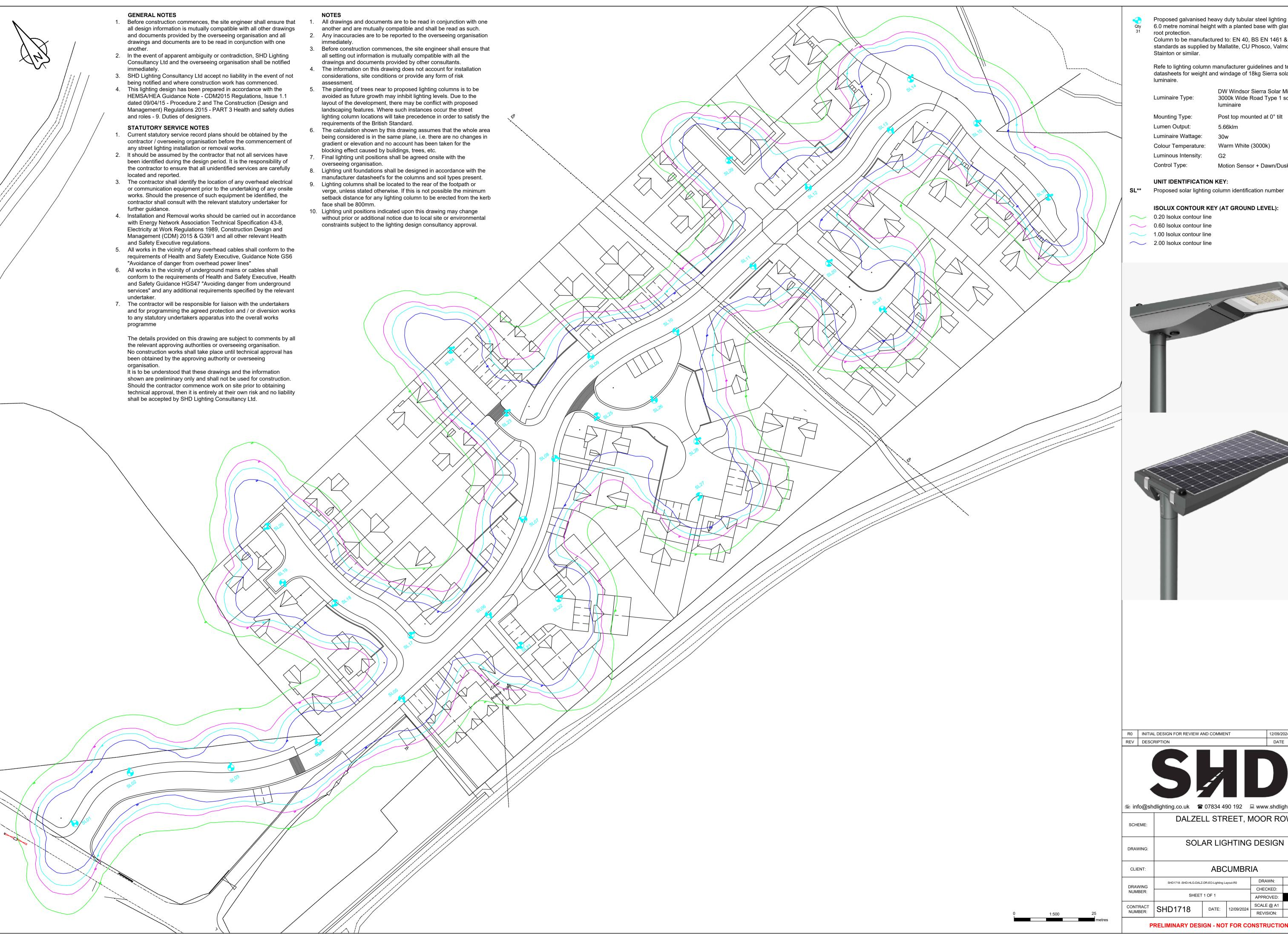
Proposed galvanised heavy duty tubular steel lighting column of 6.0 metre nominal height with a planted base with glass flake root protection. Column to be manufactured to: EN 40, BS EN 1461 & BS 5649 standards as supplied by Mallatite, CU Phosco, Valmont
