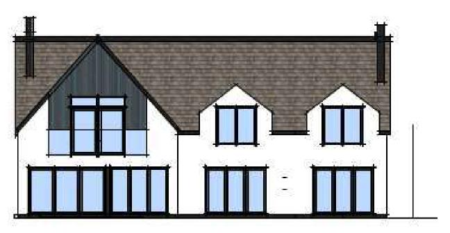
2.12 Again the low eaves can be easily rear in the building form and the windows are of a clearly dormer construction.
