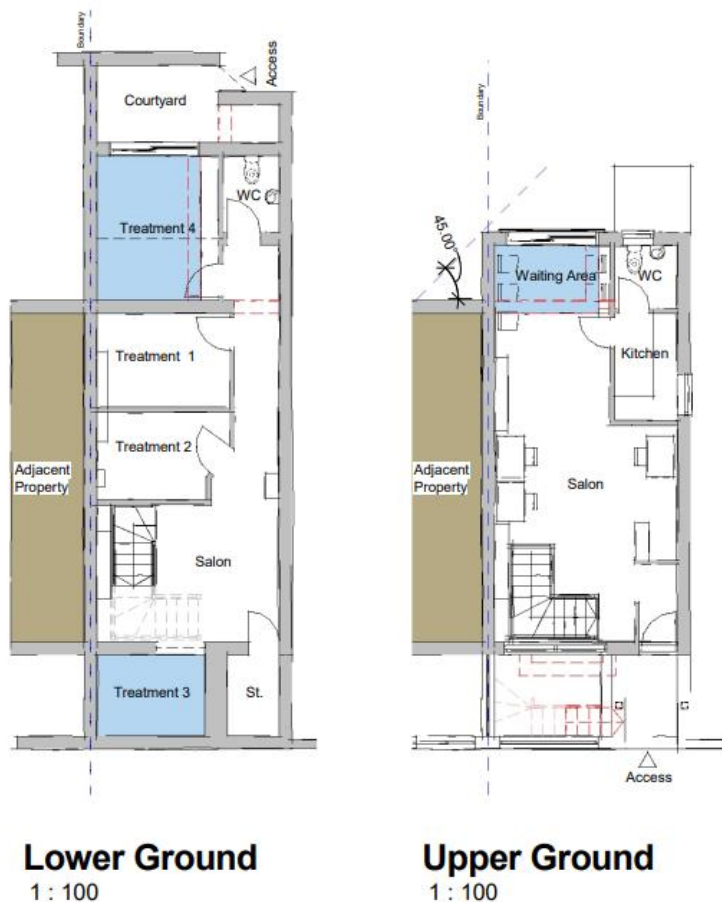
(Fig.18 – Extract of drawing 21-47-P-02 – Plans as Proposed showing the internal layout)
