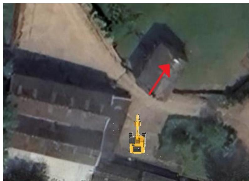
Utilising the selector grab the Machine operative will remove the roof and place straight into the lay down area ready for removal from site. Once the roof is removed the machine
