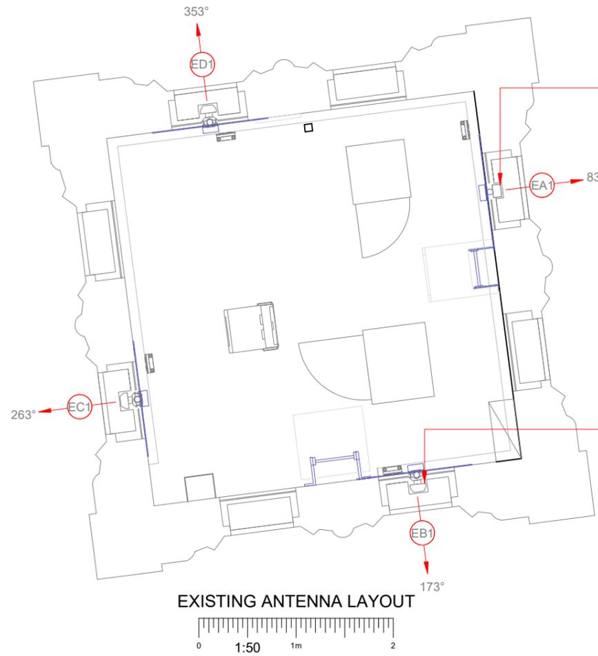
EXISTING EE 1No. CSA CS0401A ANTENNA ON EXISTING POLE MOUNTED BEHIND EXISTING GRP LOUVRE IN TOWER WINDOW. WITH 1No COMMSCOPE E15S09P75 1800 MHA FIXED TO EXISTING CABLE TRAY.
