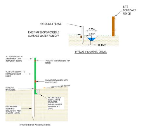
Channels should have a longitudinal gradient of no less than 1:100 towards the outlet, be vegetated as soon as practical to assist with reducing flow velocity and sediment removal, and discharge into a silt trap prior to a connection to the downstream surface water network.
