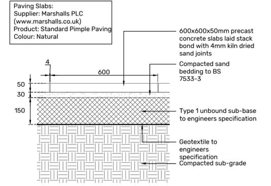
04 Concrete Slab Paving - Typical Section
