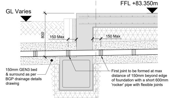
Typical Detail showing Pipe passing over Ground Beam Foundation
