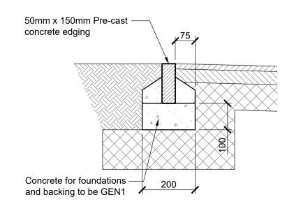
Pin Kerb Detail - (PK) Scale 1:10
