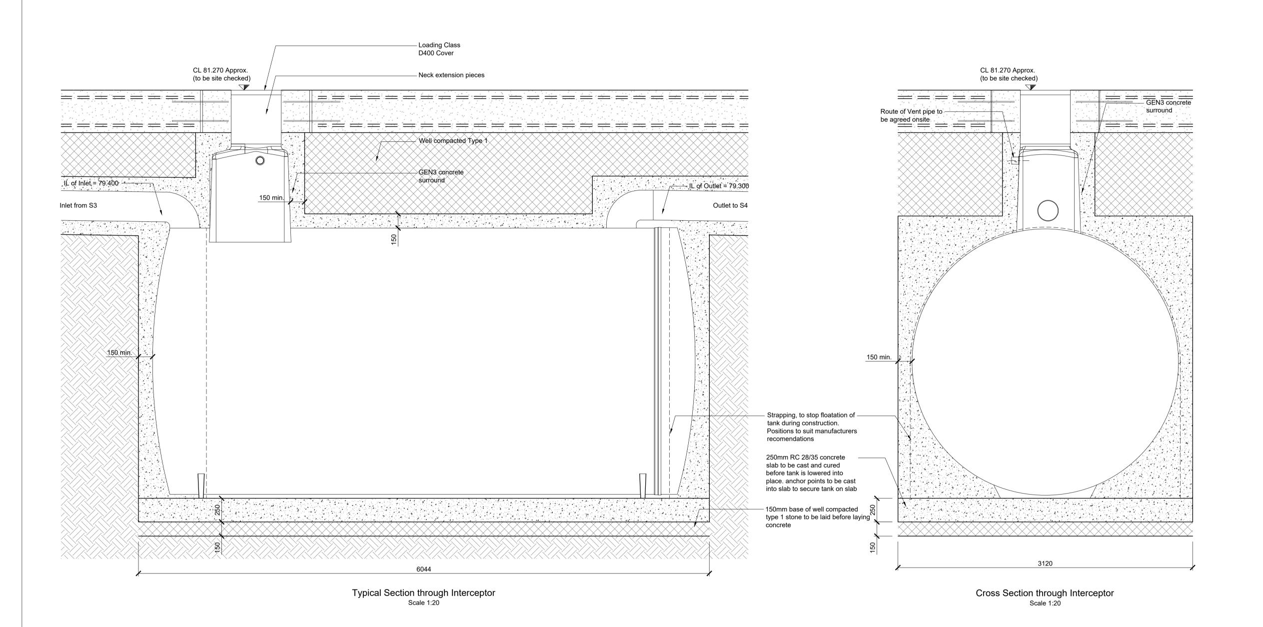
Note: Tank to be filled with water at same rate as pouring concrete to avoid floatation.
