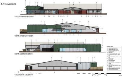
The proposed wall cladding product is Kingspan KS1000MR (micro-rib) panel – vertically fixed - Core thickness – 80mm Quadcore <u>QuadCore AWP LEC Wall Panel | Kingspan GB</u>
