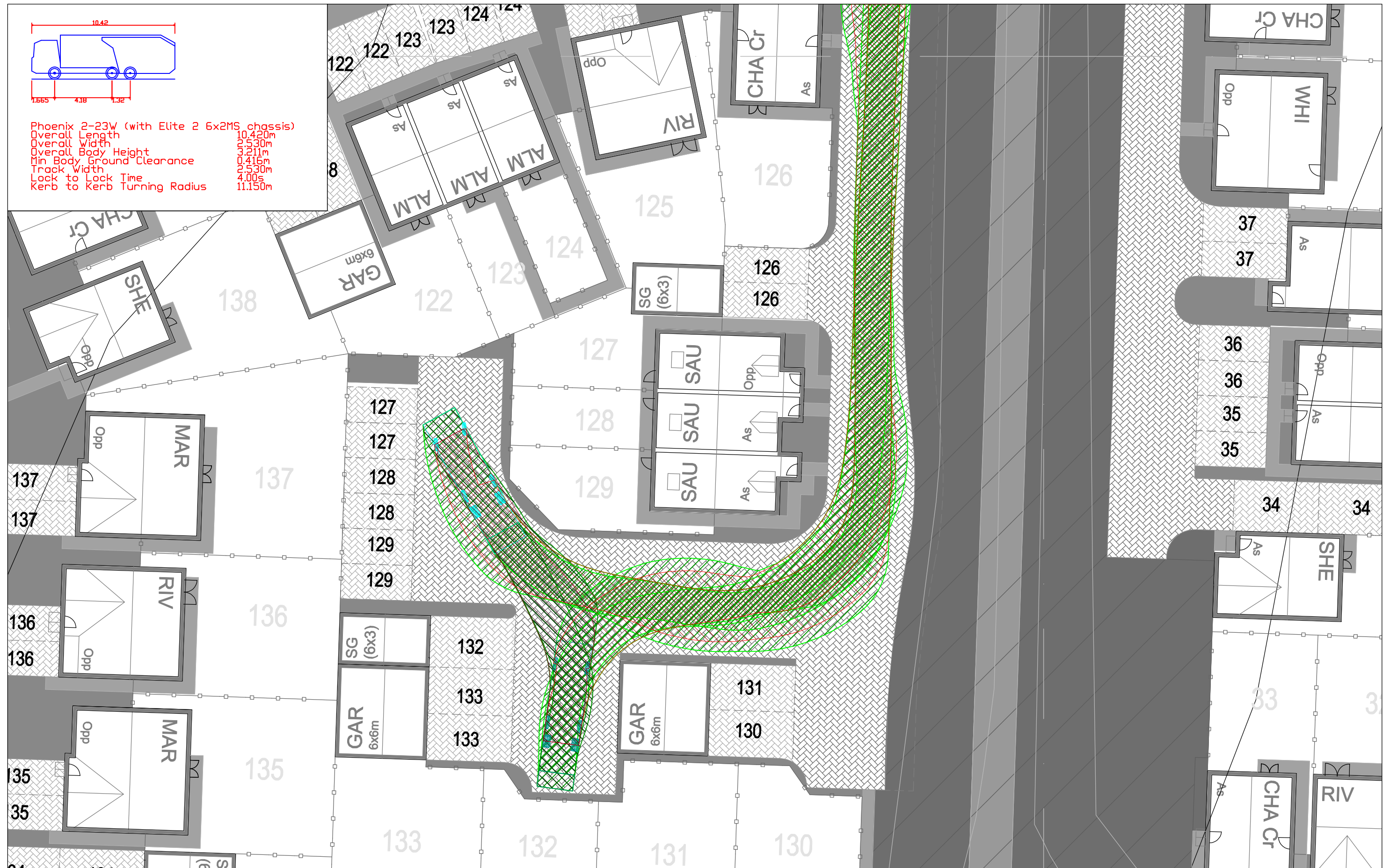
Figure A Swept Path Analysis: Large Refuse Vehicle Turning in Turning Head at Plots 127 to 133 (1:250 @ A3)
