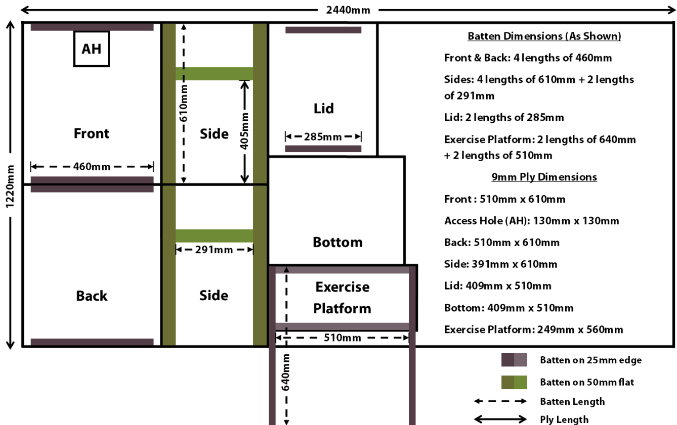
Figure 1. Diagram illustrating ply cutting plan, batten placement and corresponding dimensions.
