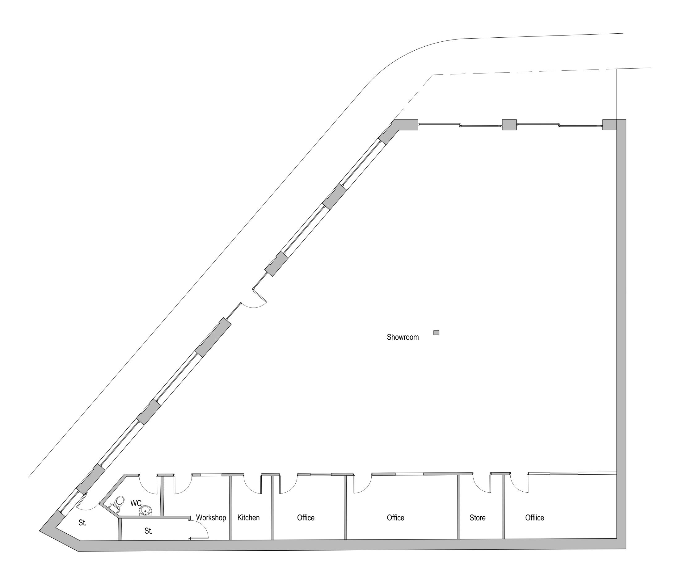
Existing ground floor plan.1:50 scale
