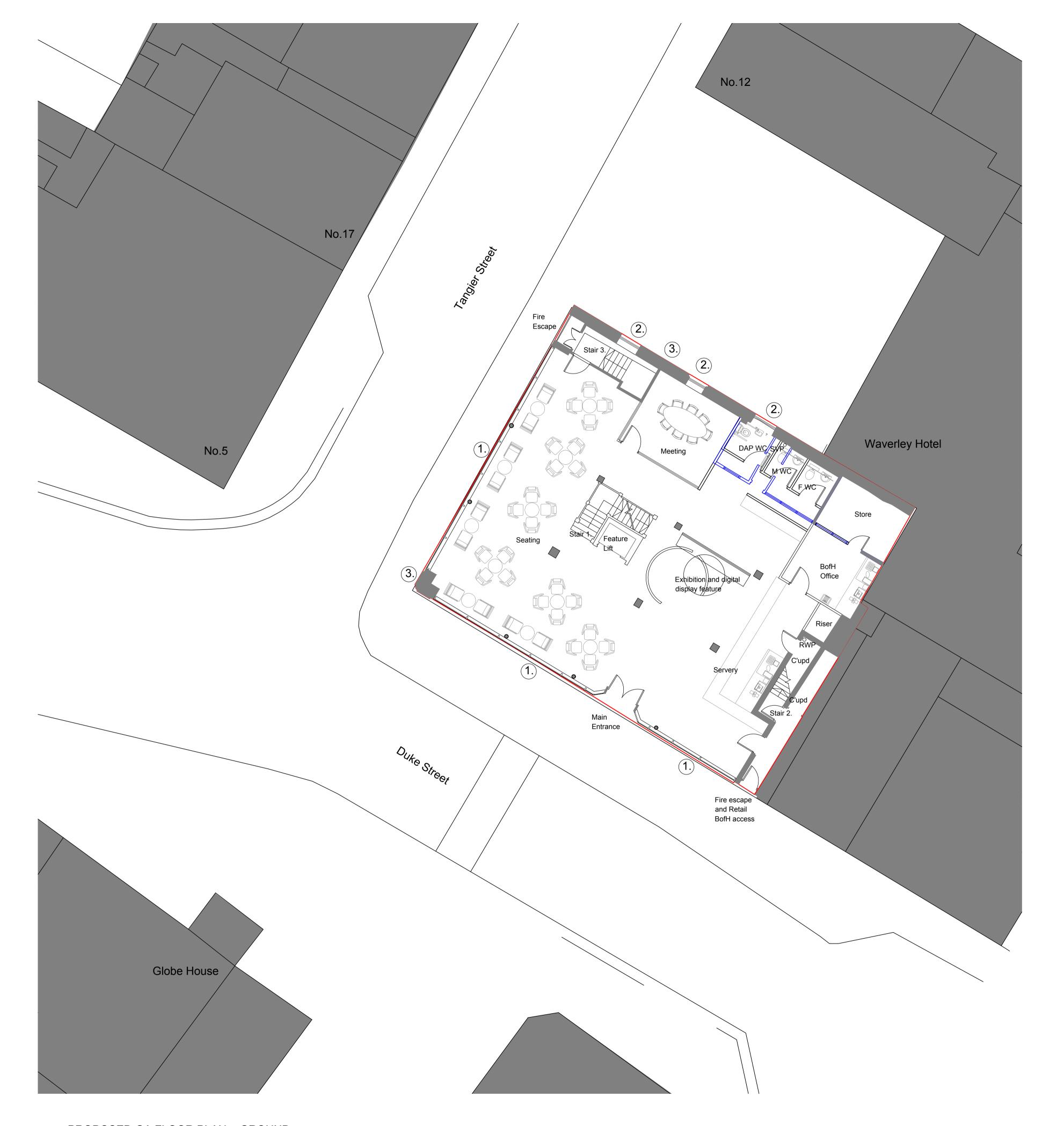
PROPOSED GA FLOOR PLAN - GROUND scale 1:100
