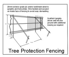
This is to be provided by Braced Heras Fencing or solid panels. Post-holes shall be excavated by powered hand auger or low ground-pressure plant working of ground protection or outside the Precautionary Zone. Alternative more traditional post supports such as the Heras Steadfast system with an additional brace can be used where this can be pinned
