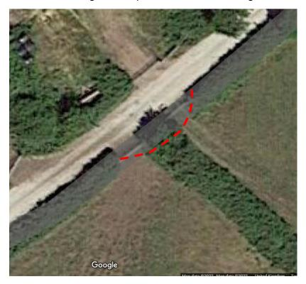
3m of the dyke kest was removed in order to set both the application site gate and the adjacent agricultural field access back as indicated on the images below and the block plan. The area was then laid with hardcore. This was to improve accesses to the fields for the larger agricultural vehicles.
