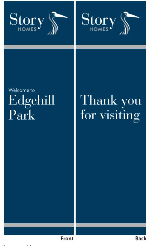
1 No. 1200mm x 4000mm Digitally printed Aluminium composite assembly having a clear protective over-laminate, internal sub-frame to be of timber construction.
