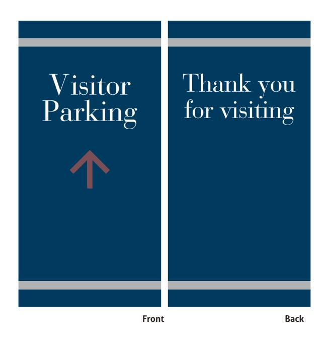
1 No. 600mm x 1200mm Digitally printed Aluminium composite assembly having a clear protective over-laminate, internal sub-frame to be of timber construction.
