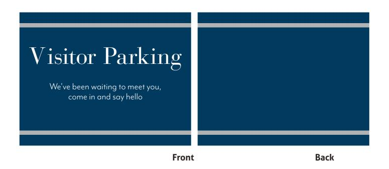
1 No. 900mm x 700mm Digitally printed Aluminium composite assembly having a clear protective over-laminate, internal sub-frame to be of timber construction.
