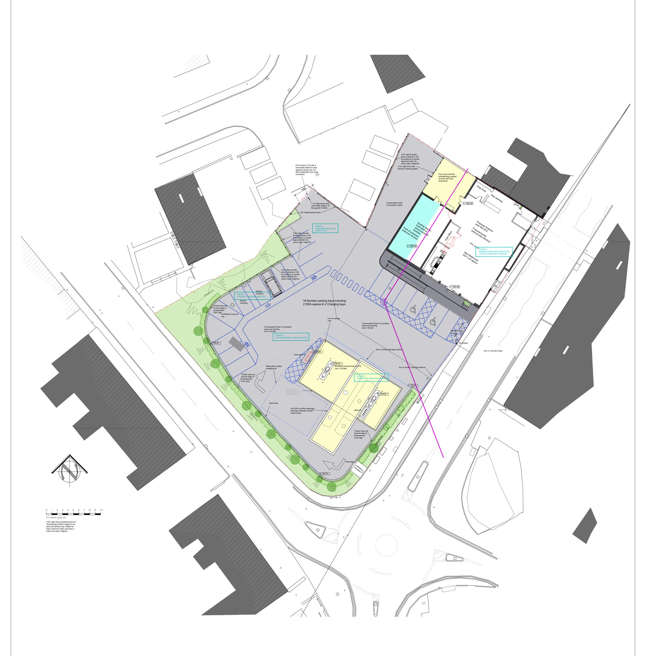
P9 Feb 2024 EVA access 3.7m with a removable bollard to stop general vehicle use, but allow pedestrian and cycle movement
