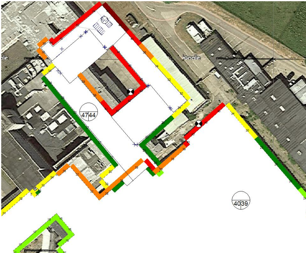
Figure 7 – Predicted noise levels at the hospital buildings
