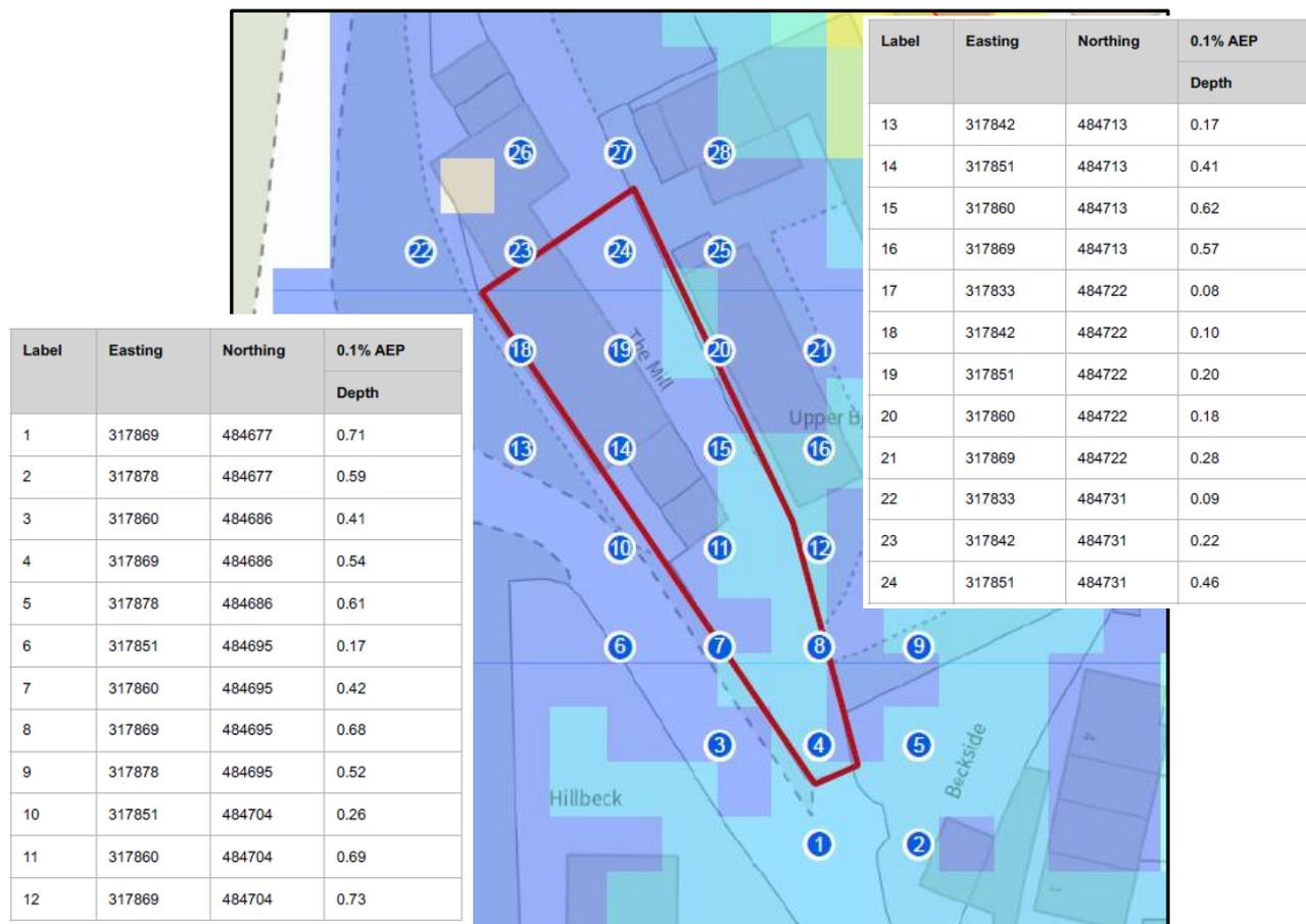
Figure 6 - Modelled 2D Fluvial Storm Extents - 0.1% AEP (Source: Product 4)
