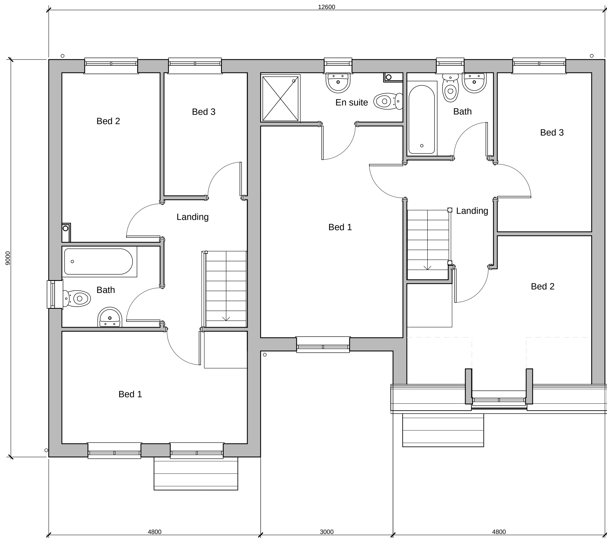
First Floor Plan Layout 1:50 @ A1
