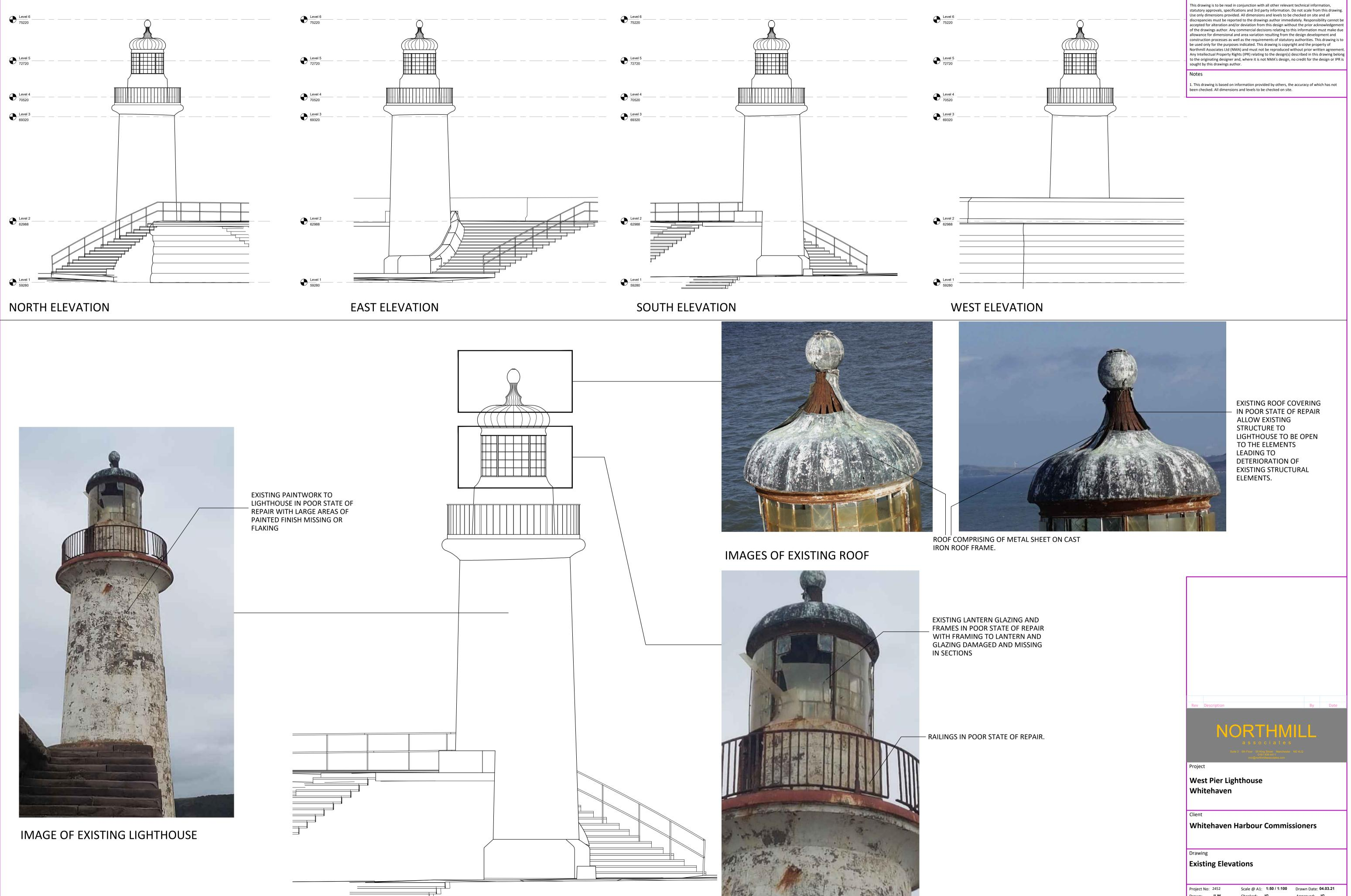
EXISTING ELEVATION SHOWING EXISTING DEFECTS (SCALE 1:50)
