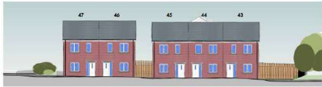
Material Option 2 - Brickwork
