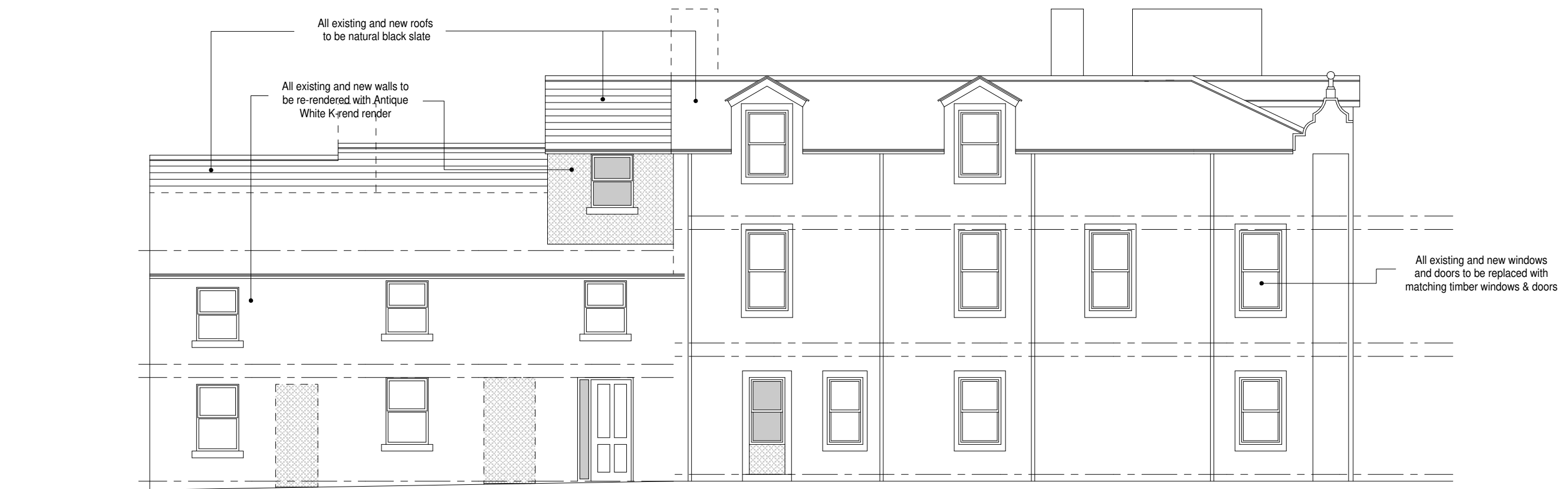
Proposed West Elevation (scale 1:100@A3)
