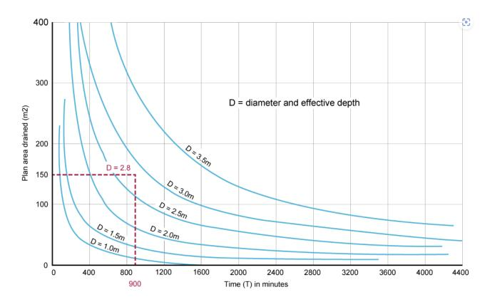
Surface area to be drained – approx. 150sq.m Three soakaways – each to hold discharge from 50sq.m Percolation test result to soakaway – 350 minutes
