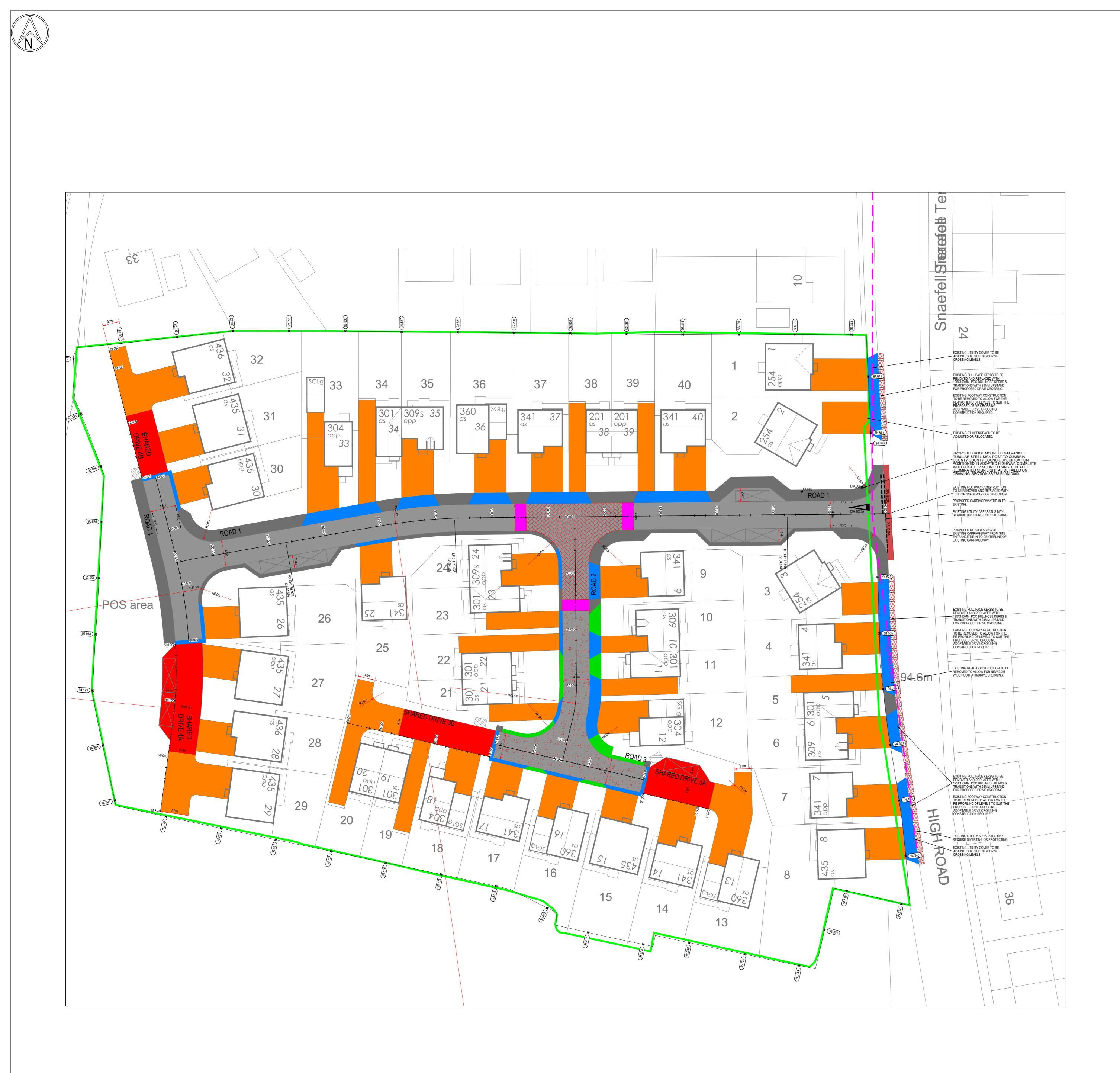
ROAD MARKING INFORMATION DIAGRAM REFERENCES RELATE TO THE TRAFFIC SIGNS MANUAL CHAPTER 5: ROAD MARKINGS ALL WHITE LINING AND ROAD MARKINGS ARE TO BE IN ACCORDANCE WITH THE CURRENT EDITION OF THE TRAFFIC SIGNS MANUAL. DIAGRAM 1003A: MARK=0.6m, GAP=0.3m, WIDTH=0.2m
