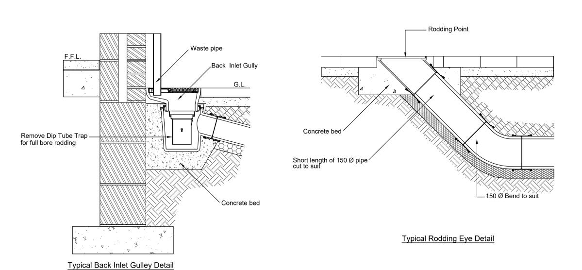
All work undertaken in accordance with sewers for adoption 6th edition "A Design & Construction Guide For Developers" This drawing is protected by copyright and must not be copied or reproduced without the written consent of M&P Gadsden Consulting Engineers Ltd. No dimensions are to be scaled from this drawing. All dimensions and sizes to be checked on site. © Rev. Date. Notes. Client/Project.
