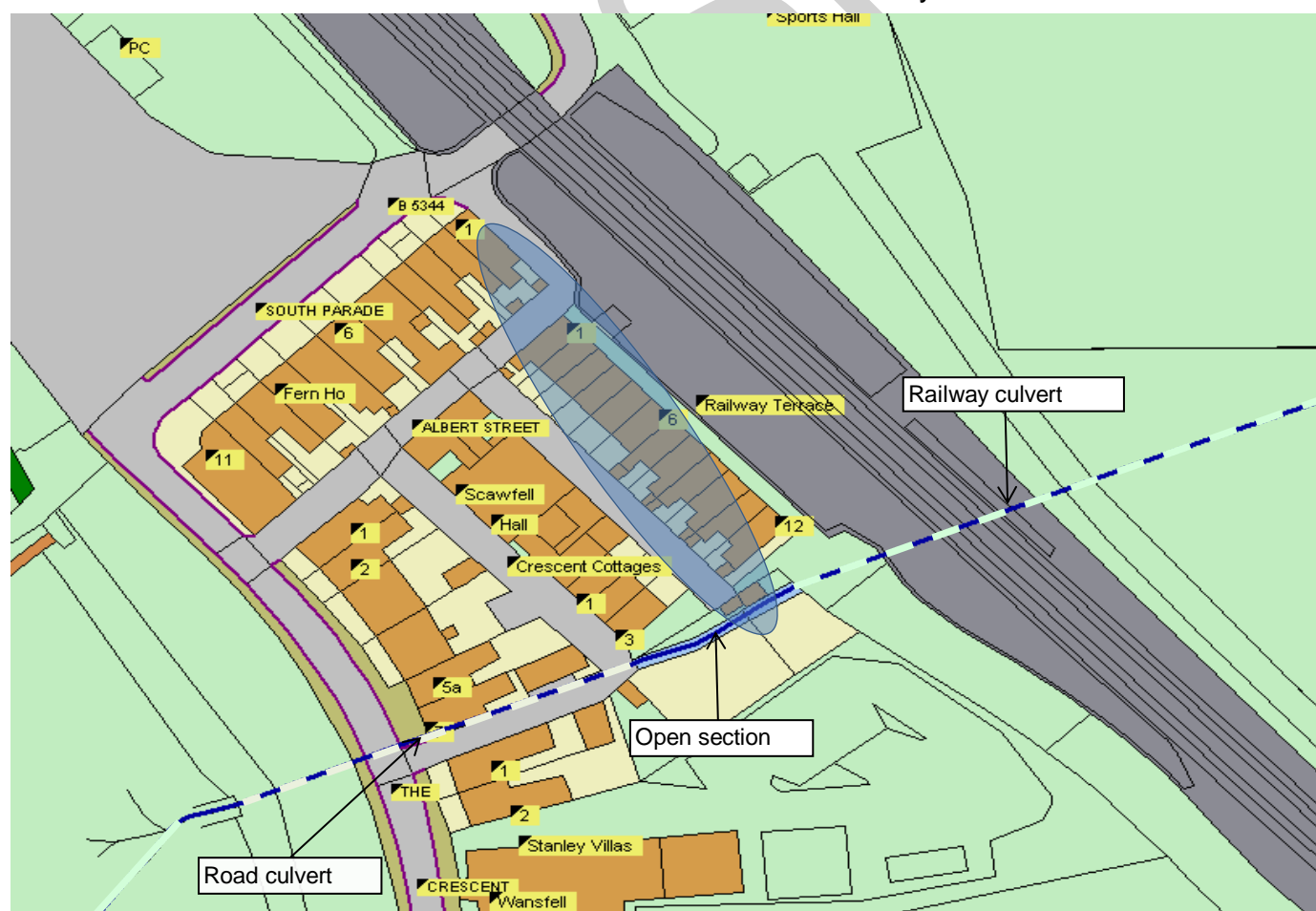
Figure 5 Plan of the Railway Terrace and Albert Street area showing the line of the culverts and the location of the flooding.
