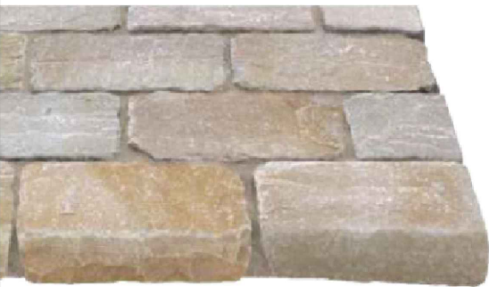
Hard Surface 3 : Marshalls natural stone sets 'split and tumbled, Autumn Bronze' 200mmx100mmx50mm with Marshalls Cropped Granite Eclipse Setts 100x100x100m forming border.
