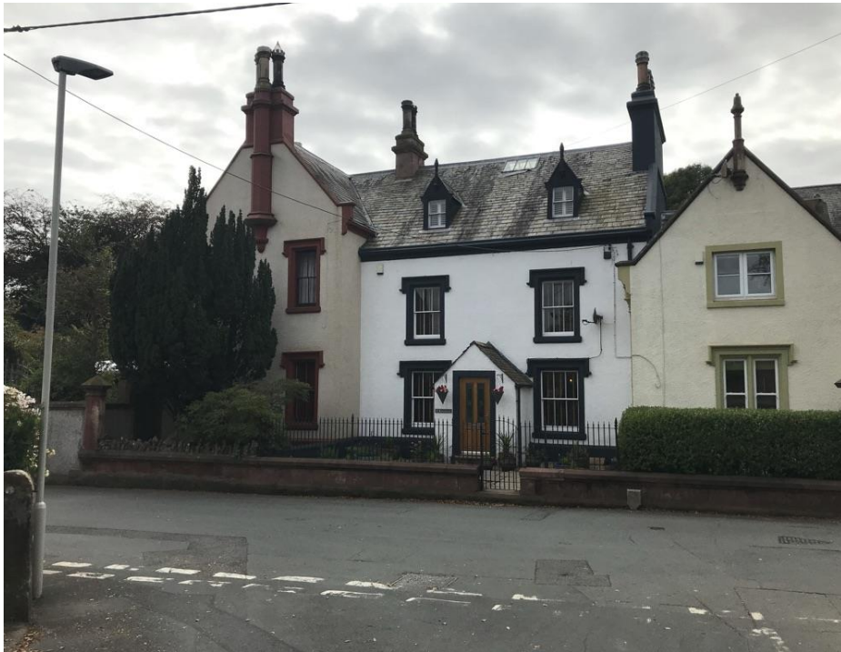
Main House ( now subdivided ) at Barwickstead - high level rooflight on main house replicated on barn with less formality - proposed use of dormers not appropriate for a conversion scheme.
