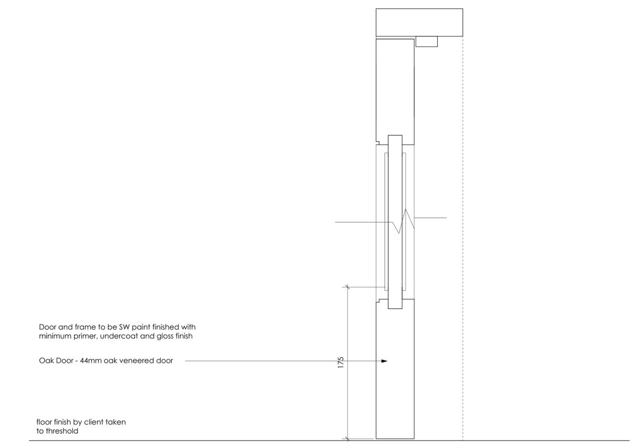
TYPICAL INTERNAL OAK DOOR SECTION Scale 1 : 2
