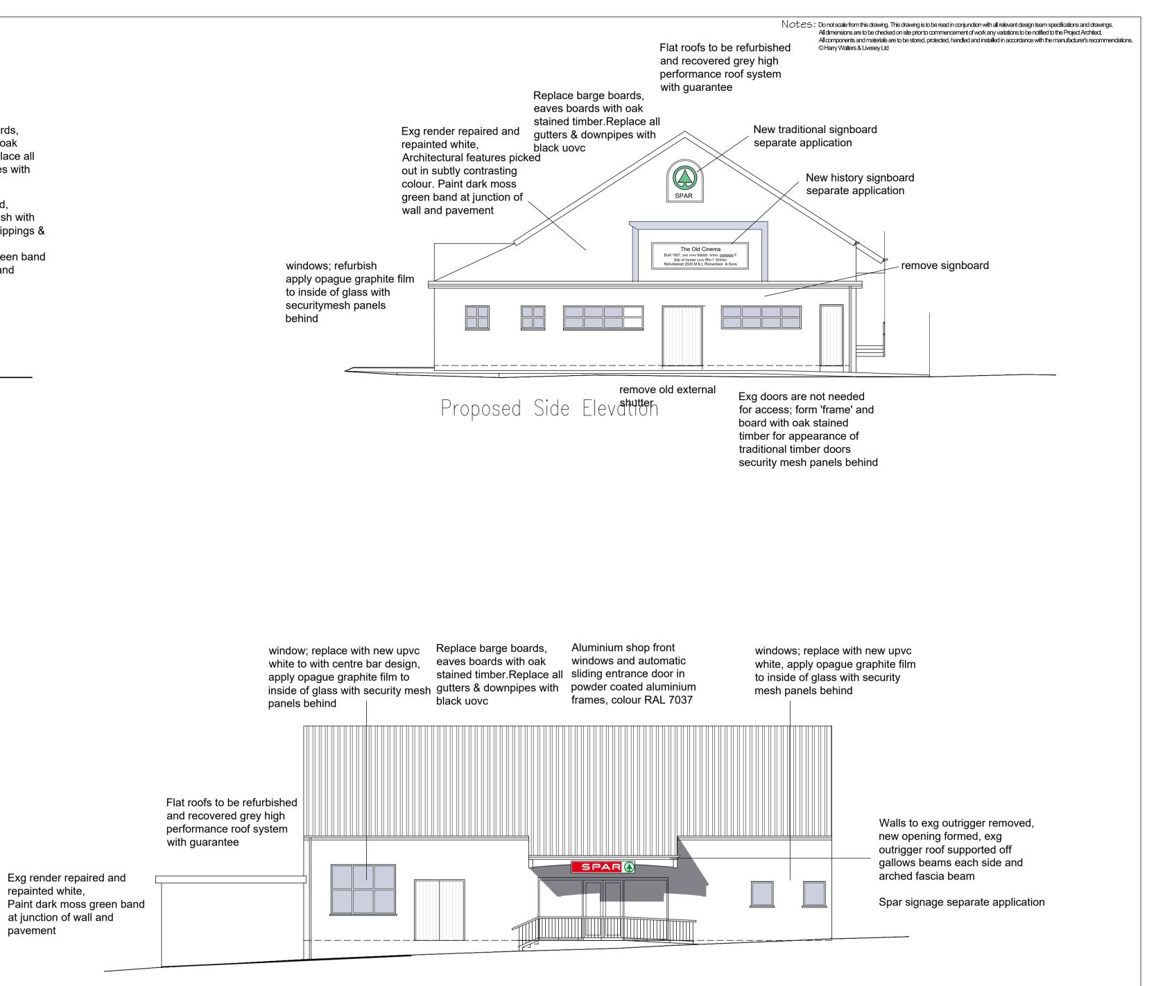
Exg door is not needed for access; Proposed Front Elevation form 'frame' and board with oak stained timber for appearance of traditional timber doors security mesh panels behind. Remove shutter and steps c/w
