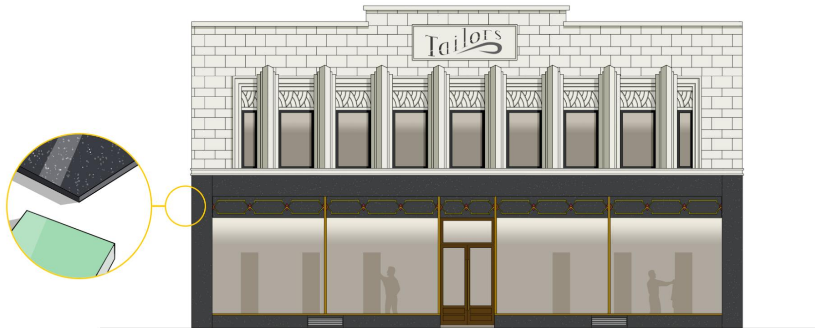
Figure 4 An Art deco style building, which might have been built in the 1930s. Interwar cladding (faience, Vitrolite glass, granite etc.) is fragile and often difficult to repair/replace, so great care should be taken with it.
