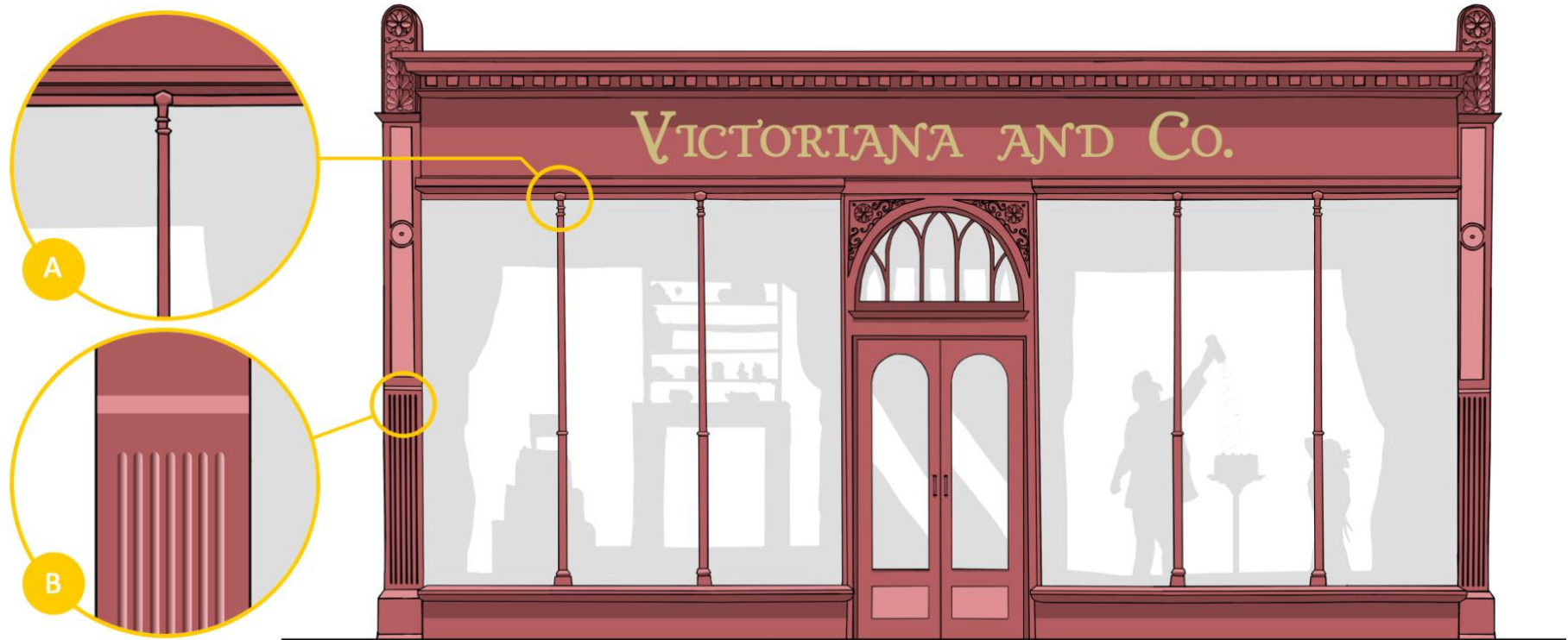
Figure 2 A Victorian style shopfront reminiscent of the latter 19th century. (A) An iron colonette serving as a mullion; (B) The pilaster is fluted, meaning it has grooves that introduce rhythm and lightness
