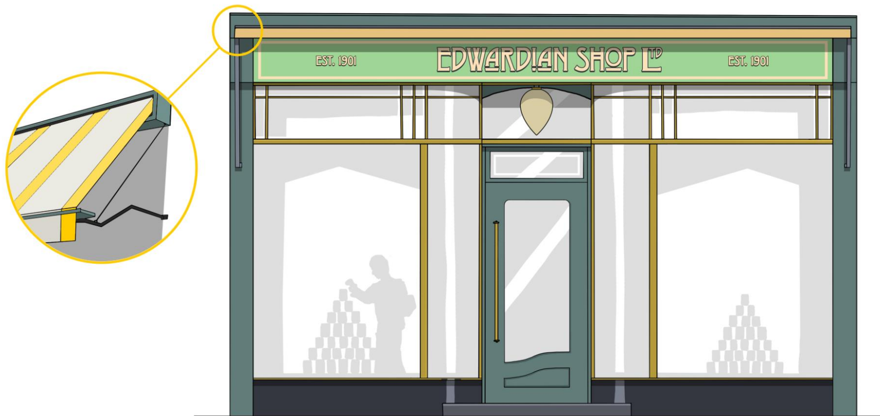
Figure 3 An Edwardian style shopfront with retractable blind. You may wish to consider incorporating a blind of this design on your own shop.
