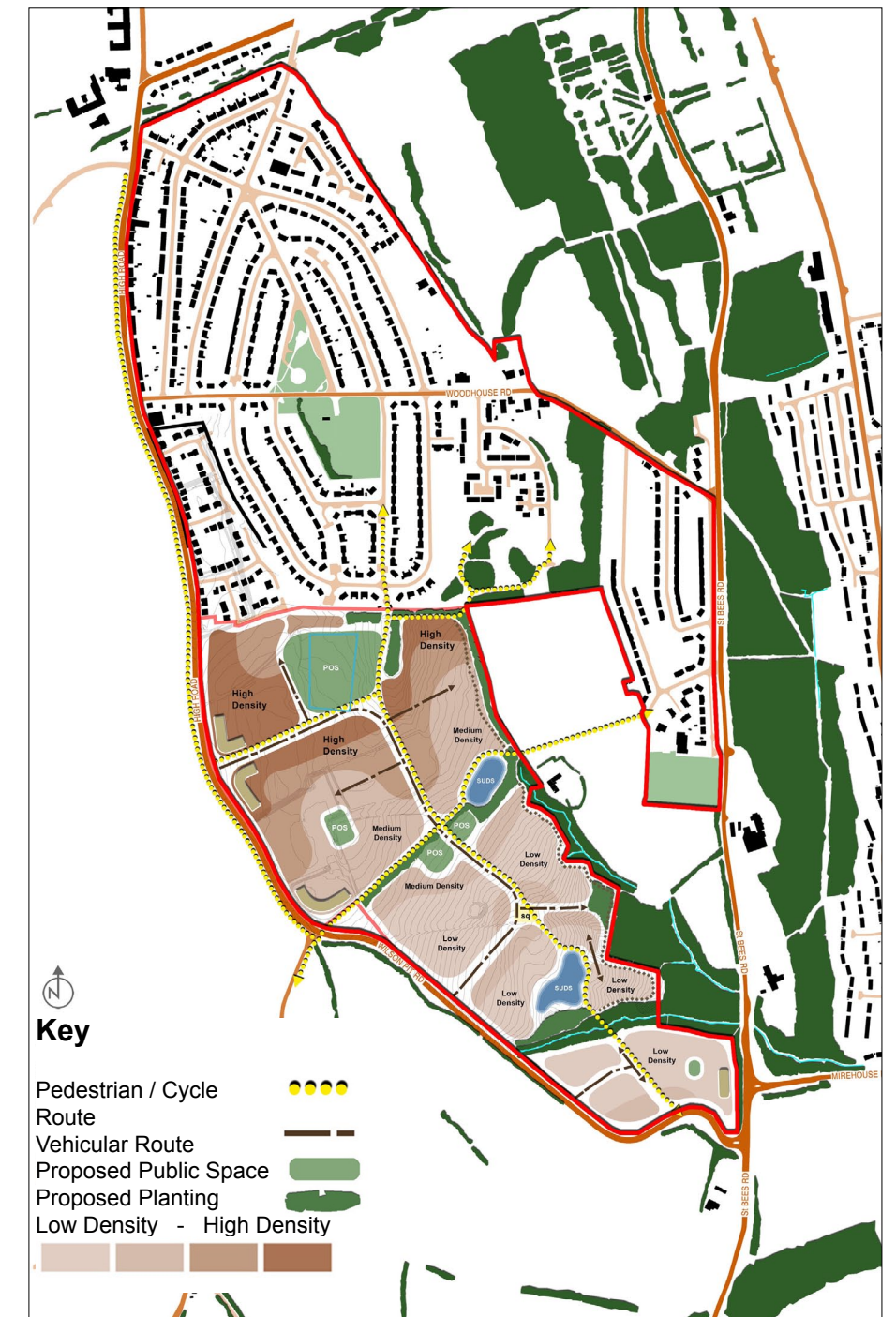
Plan 3 - The main focal point and highest density areas are positioned at the Northern part of the scheme next to the main access point, Woodhouse Estate boundary and the main Public Open Space. As the development flows down the hill to the South the density levels decrease and dwelling sizes increase creating pockets of executive housing
