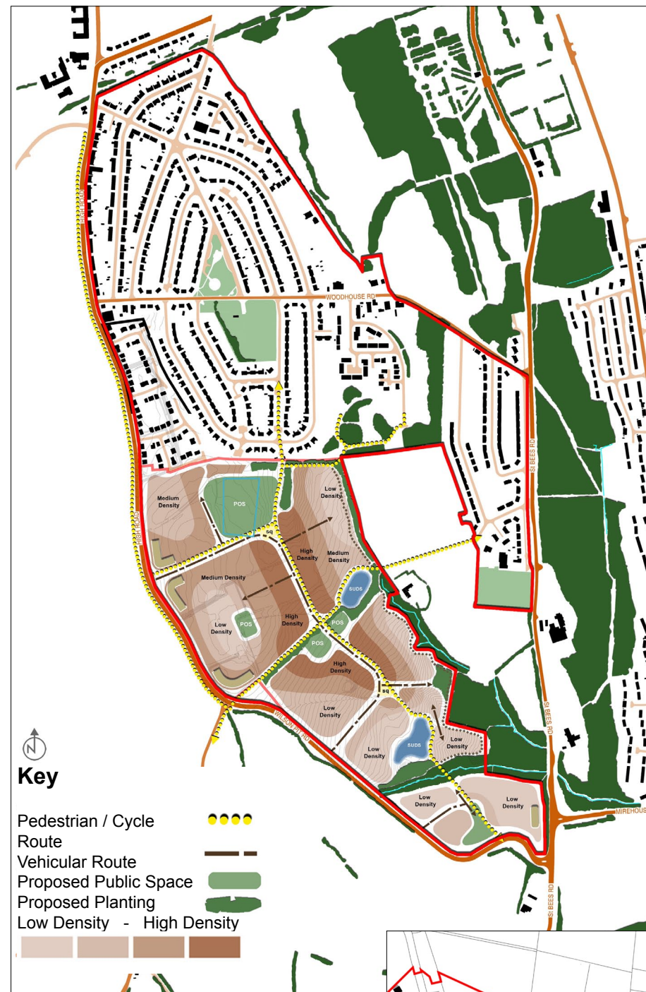
Plan 2 - The development focuses on a higher density street as a focal point running North South from the main Public Open Space area to the lower area of the scheme. This allows the development of a scheme which will reflect both Whitehaven and its outlying villages in terms of its layout and the look of the houses.
