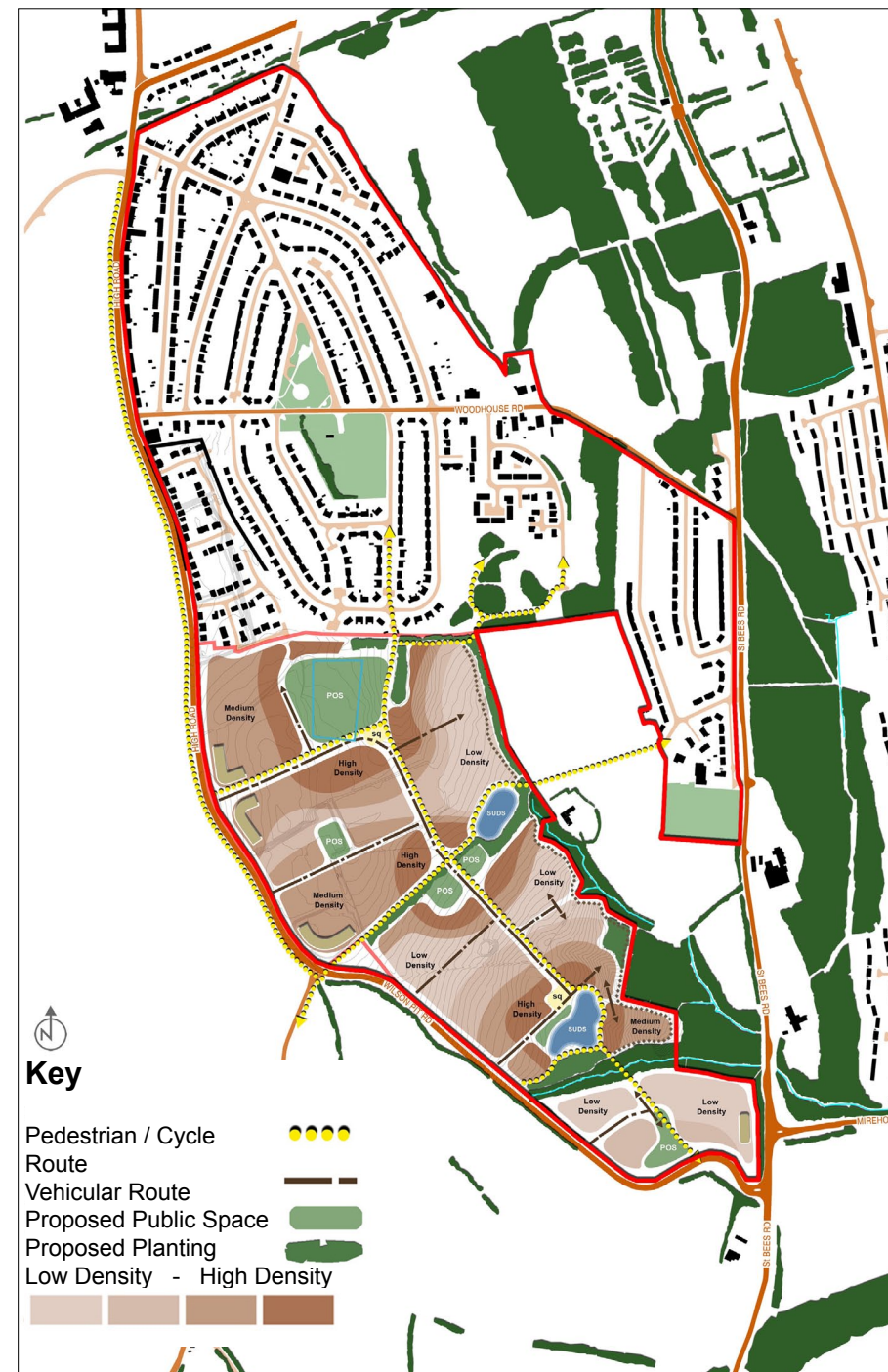
Plan 3 - The scheme has 3 main smaller focal points at key intersections of Public Open Space, existing Landscape Features and SUDS ponds. This helps break up the scheme into smaller elements each with their own focal point
