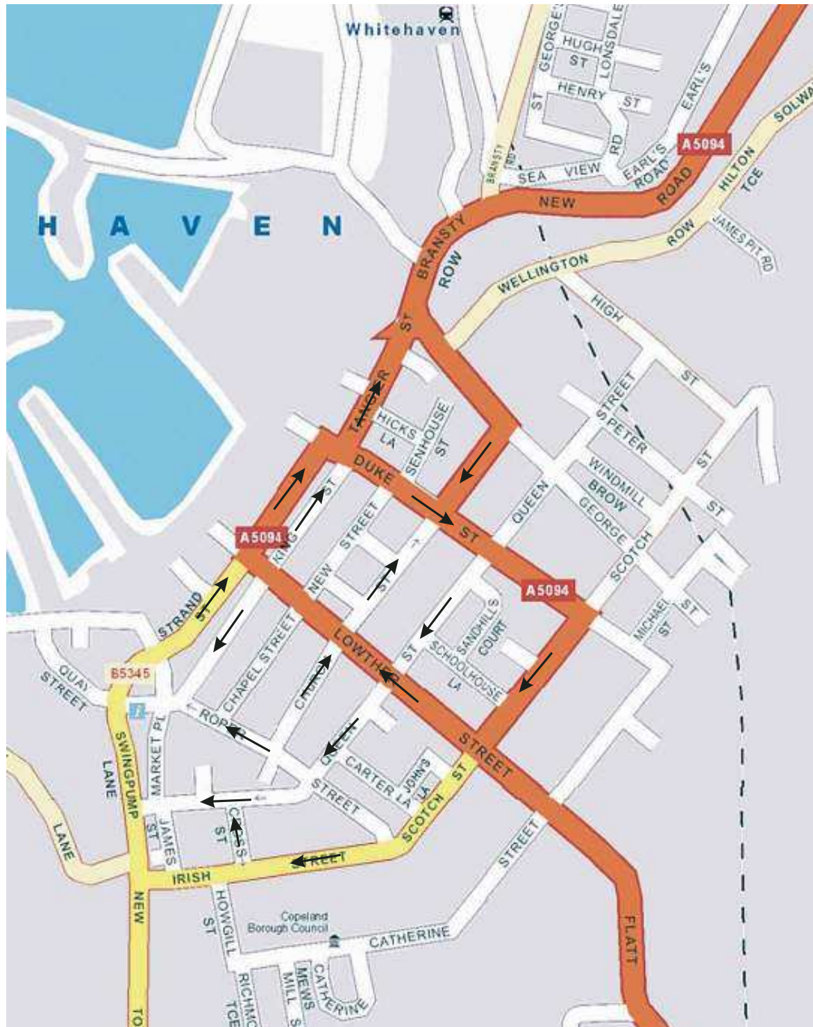
Figure 7.2: Road Network and One Way System
