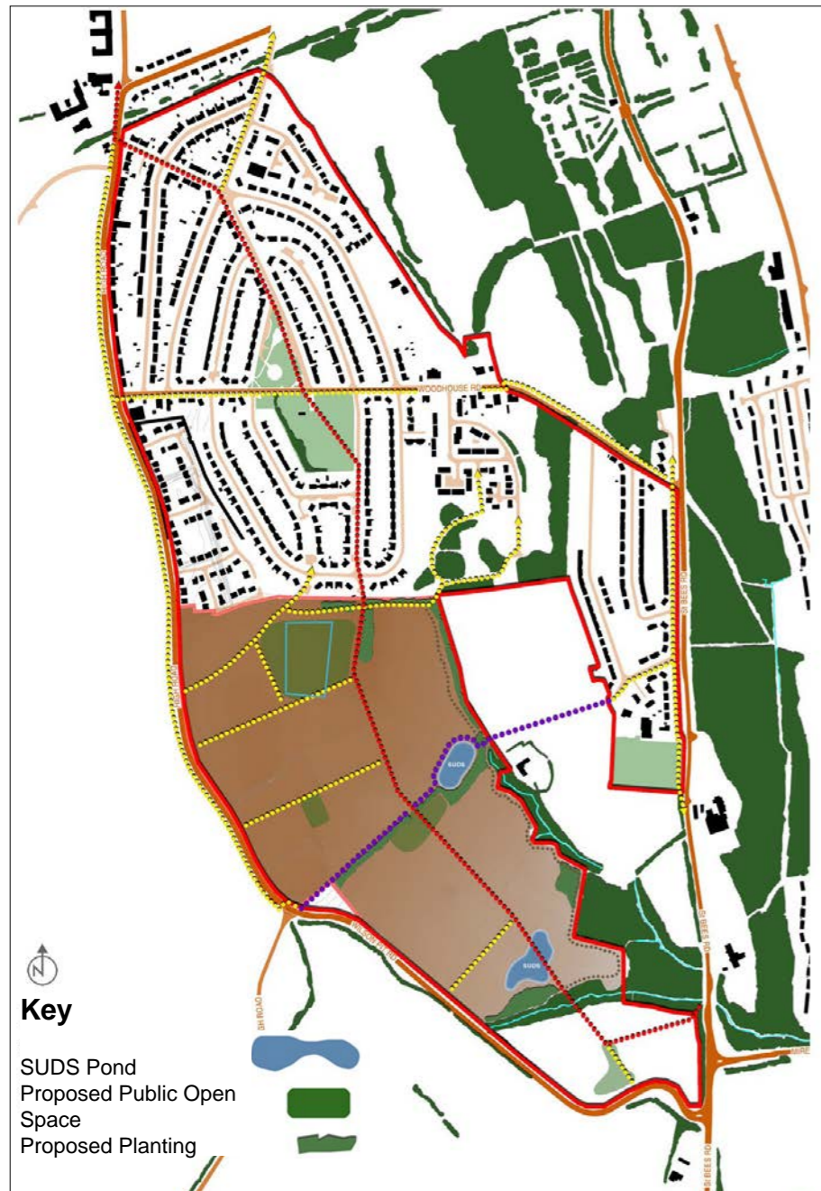
Plan 8 - Topography, key proposed structural landscaping areas, SUDS areas (Sustainable Urban Drainage System) and pedestrian connectivity
